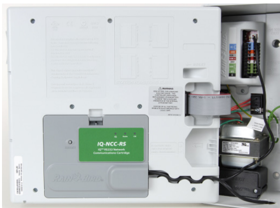
IQ Communication Cartridge (installed)
